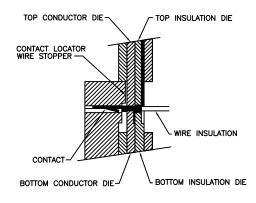
SECTION THROUGH DIE NEST WITH CONTACT IN POSITION
